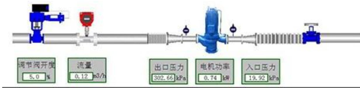
$$\eta_{\text{泵}} = \frac{G \times H \times 9.81 \times 1000}{P \times 1000 \times 3600} = 0.00273 \frac{G \times H}{P}$$
